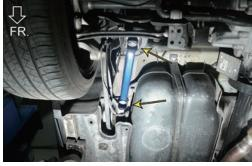
2. Install **Brace** to the vehicle, then reinstall the bolts to secure the brace. 安裝 **結構桿** · 並鎖回螺絲以將桿身固定。
